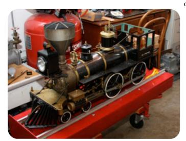
one side of the shop sits the coal fired Governor Stanford live steam locomotive with it's hundreds of hand built pieces assembled into an operating replica of the historic machine. In the middle, there is a Shay locomotive under construction with it's exposed gearing all meticulously cut
