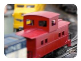
Cupola on steroids? Well, sort of. Alan Teruya raised the roof on this caboose in order to install an onboard camera. As the train rolled around Michael's layout we got a conductor's eye view of the action on Alan's notebook computer. A red light on the back of the caboose indicates that the camera is turned on. Reversing the caboose in the line up allowed us to watch as a second locomotive that was chasing us on the main line closed the gap.
